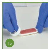
Obtain samples from surfaces, liquids, personnel, swabs and the air (using our unique magnetic dip-slide holder)
