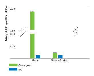
Comparison of reactivity towards glucans between kinetic chromogenic LAL and rFC. The false positive signal from the LAL assay is reduced in the presence of a glucan blocker. rFC does not detect any glucan activity; it is endotoxin-specific.
