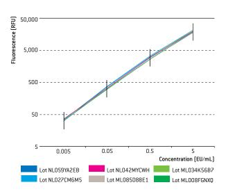
Endotoxin standard curves using 6 different lots of rFC. The log net fluorescence is proportional to the log endotoxin concentration and is linear in the 0.005 - 5 EU/mL range. Lot-to-lot standard curves exhibit excellent reproducibility.
