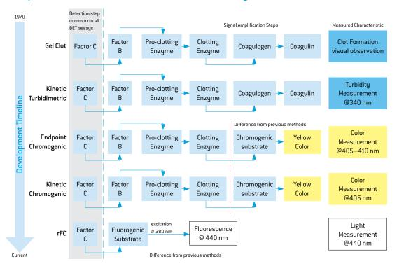
rFC is the same binding protein operating in the LAL assay. The activated recombinant Factor C enzyme cleaves a substrate directly instead of activating another enzyme in a series (the LAL cascade). The substrate has a fluorescent tag, which gives a wide dynamic range with better resolution.
