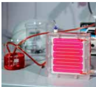
Vivaflow 200 set-up for diafiltration
