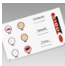
O.B.I.S. test card w/ positive reactions.
