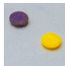
Beta Lactam Reagent Disk w/negative test (top) and positive test (bottom).
