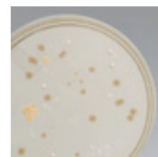
Tryptic Soy Agar Settling Plate w/growth.
