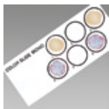
Color Slide II Mononucleosis test card w/positive and negative reactions.
