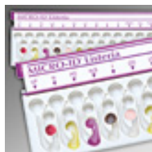
Micro-ID Listeria Identification System panel w/inoculated wells.
